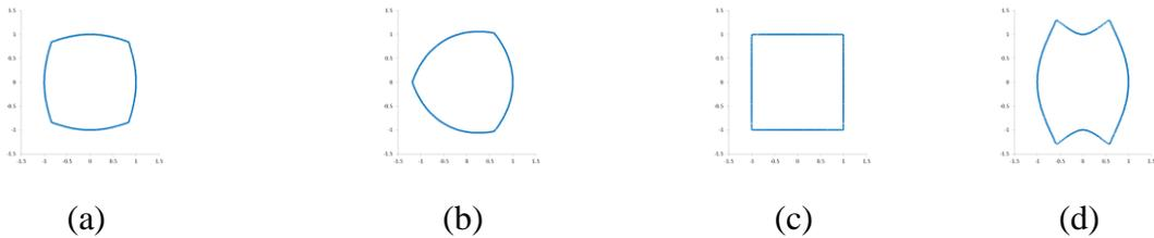
**Figure 1** Examples for different Superellipse parameters (a) [ $a=1, b=1, m=4, n_1=200, n_2=100, n_3=100$ ]; (b) [ $a=1, b=1, m=3, n_1=200, n_2=100, n_3=100$ ]; (c) [ $a=1, b=1, m=4, n_1=100, n_2=100, n_3=100$ ]; (d) [ $a=1, b=1, m=4, n_1=50, n_2=20, n_3=200$ ]
