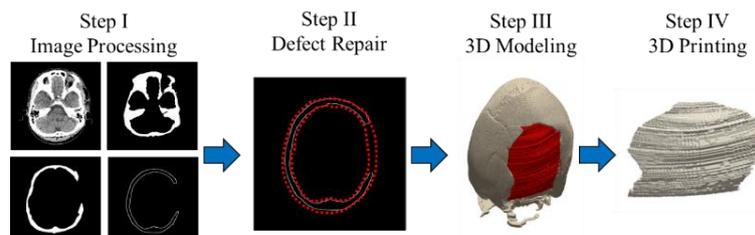
**Figure 2 Main steps of the prosthesis reconstruction procedure**
