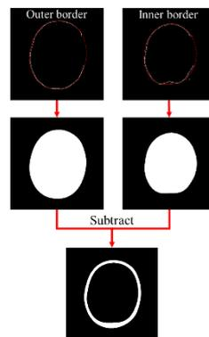
**Figure 5 Thickness trimming procedure for every CT layer**
